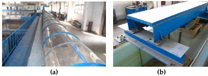
Figure 1. Equipment for the wave cross-sectional model test. (a) Multifunctional wave test flume. (b) Absorbing wave generator.
