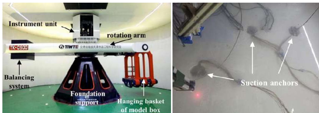
Fig. 1 The geotechnical centrifuge and model suction anchors
