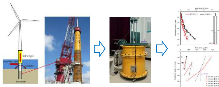
Fig. 1 Model test of offshore wind turbine foundation
