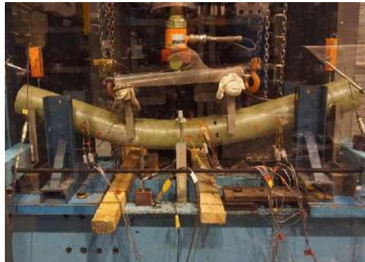
Fig. 1 Failure mode of the GFRP pile.
