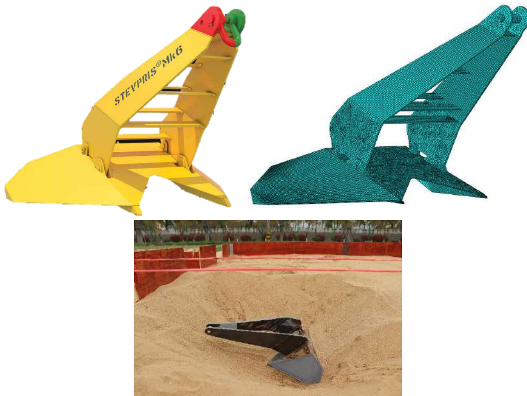
Fig. 1 Illustration of numerical and physical drag anchor models
