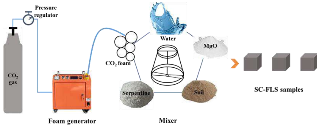
Fig. 1 Schematic diagram of samples preparation
